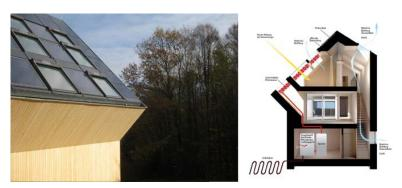
Figure 7: Velux Sunlight House, Pressbaum (Arch. Hein & Troy, A), Building integrated PV- and solar thermal technology – Functional depiction
